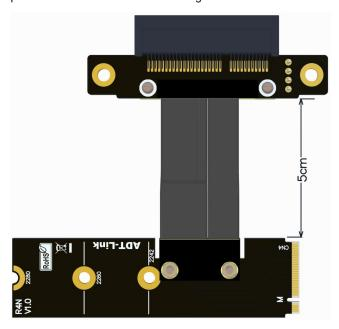
Accessories description: A SATA power adapter cable is included with the product, and it must be connected to have 12V power supply.
