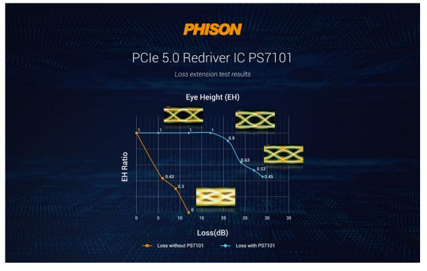
PCIe 5.0 has high requirements on the equipment. As long as the extension cable is connected, the signal will be attenuated. This product does not guarantee the full speed of PCI-E 5.0. The equipment is aging. If the signal is poor or the environment is not good, please slow down to PCIe 4.0 or lower.
