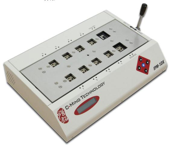
IPM-1DX e-MMC/eMCP Duplicator is designed to meet e-MMC/eMCP device content duplication/verification manufacturing needs on manual production line. IPM-1DX e-MMC/eMCP拷貝機,乃是特地針對手動產線在生產過程中,對於 e-MMC/eMCP的內容複製與內容驗證之需求而設計。
